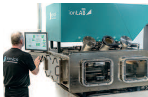
▲ ionLAB400: low pressure system equipped with ion implantation and plasma PVD technologies for flat or 3D parts treatment
